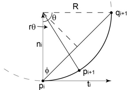
Figure 18: Computing the circular-arc connector.
