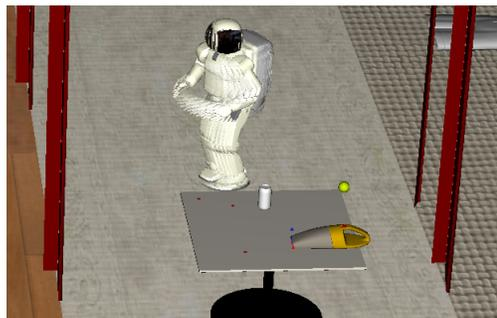
Fig. 5. Depiction of the action of the *fixate* program; the simulated robot is commanded to focus on the vacuum. The robot turns on its base while simultaneously orienting its head.
