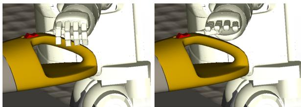
Fig. 4. Using *release* to relinquish the grip on the vacuum
