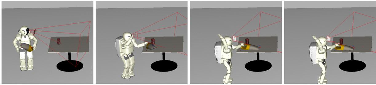
Fig. 6. Using a complex behavior composed of *fixate*, *position*, and *release* to put down an object
