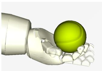
Fig. 3. Depiction of using the *grasp* program to clutch a tennis ball
