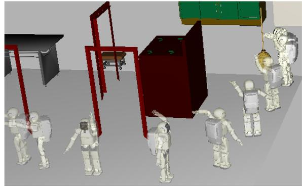
Fig. 2. A depiction of the *reach* task program in action. This figure shows the process of reaching to a broom in a simulated real-world environment in a collision-free manner.
