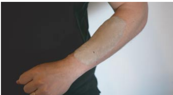
Figure 8.17 Artificial skin, created from silicon, covered the 3in3out device to simulate implantation and allow for testing. (Adapted from [26] with permission.)
