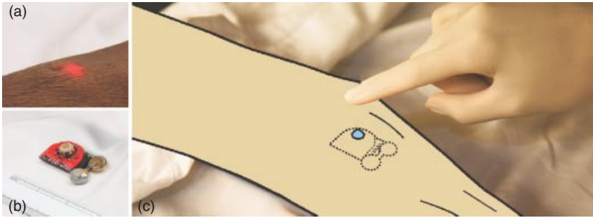
Figure 8.16 (a) Actual photograph of the LED output through the skin. (b) This standalone prototype senses input from an exposed trackball and (c) illuminates it in response. (Adapted from [26] with permission.)
