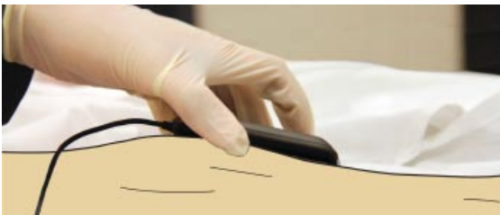
Figure 8.13 The wireless charging mat docks to the receiver, which is implanted inside the specimen. (Adapted from [26] with permission.)
