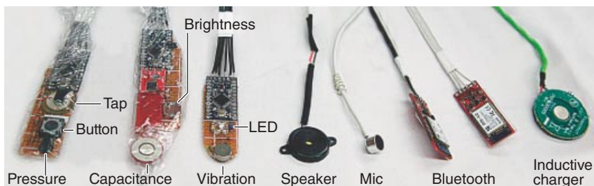
Figure 8.3 Devices implanted during the study. Plastic bags around devices prevent contact with tissue fluid. (Adapted from [26] with permission.)
