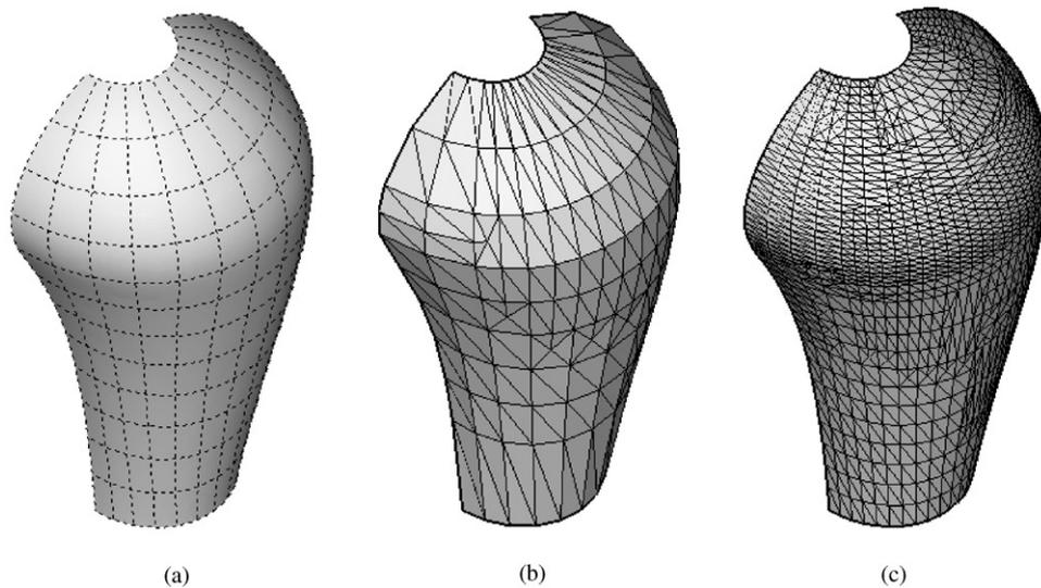
Fig. 13. Parametric-surface tessellation of gearshift-knob surface: (a) bicubic B-spline surface, resulting piecewise-planar approximants with pre-defined tolerance, (b) 1.0, and (c) 0.1.
