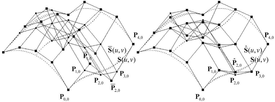
Fig. 5.  $u$ -directional stepwise degree reduction of Bezier surface of degrees (4, 4).
