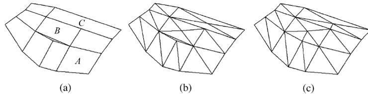
Fig. 10. Water-tight triangular net construction with proposed crack prevention method.
