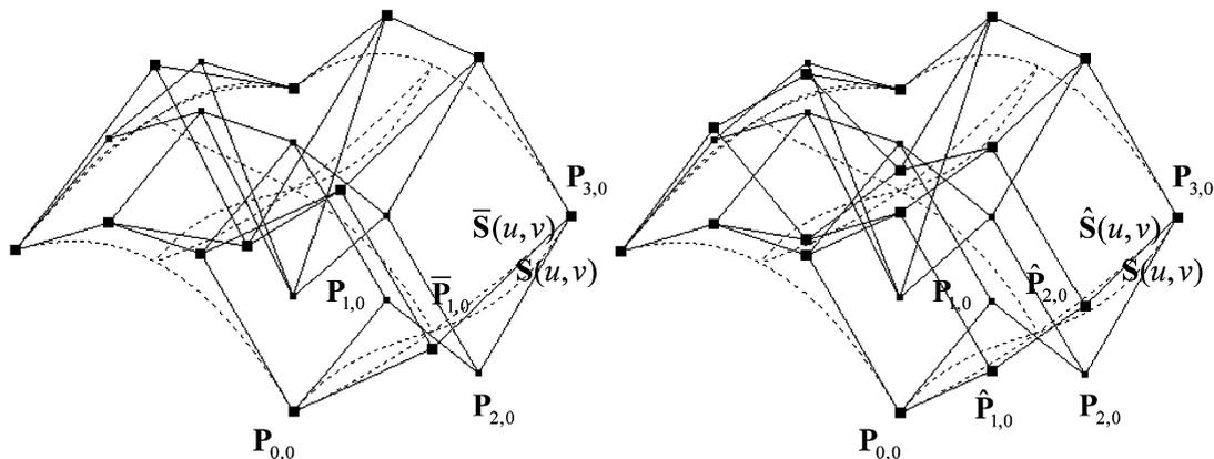
Fig. 6. *u*-directional stepwise degree reduction of Bezier surface of degrees (3, 3).
