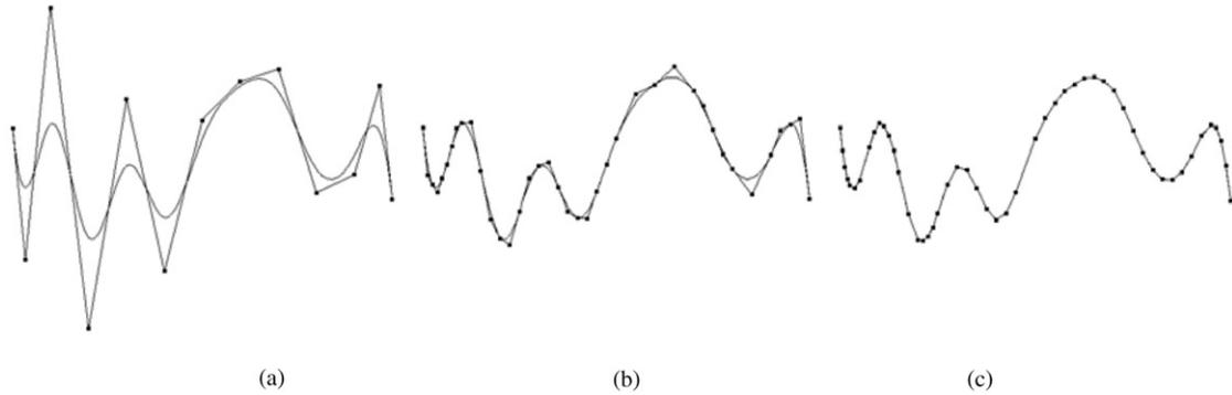
Fig. 2. Parametric-curve polygonization method based on stepwise degree reduction: (a) given cubic B-spline curve, (b) quadratic Bezier curves, and (c) resulting piecewise-linear approximant.
