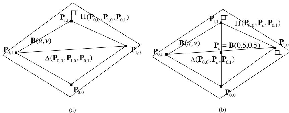
Fig. 11. Conversion of bilinear surface into triangles.
