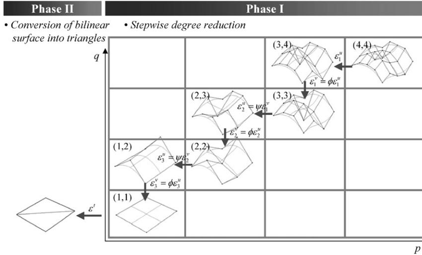
Fig. 7. Schematic diagram of exponential step-tolerance method.
