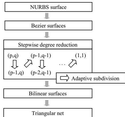
Fig. 3. Overall procedure of parametric-surface tessellation.
