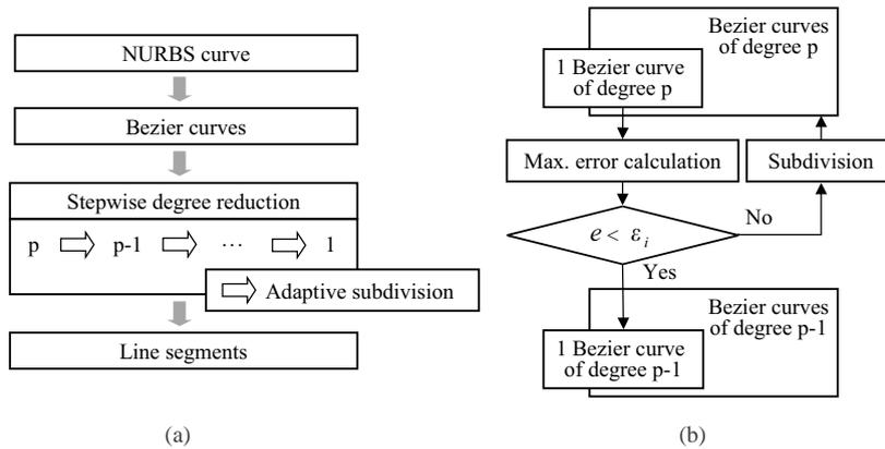
Fig. 1. Basic idea of parametric-curve polygonization: (a) overall procedure and (b) adaptive subdivision.
