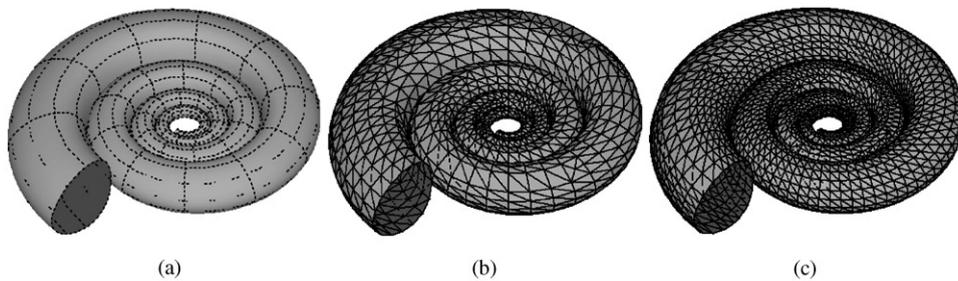
Fig. 12. Parametric-surface tessellation of nautilus-shell shaped surface: (a) bicubic B-spline surface, resulting piecewise-planar approximants with pre-defined tolerance, (b) 2.0, and (c) 1.0.
