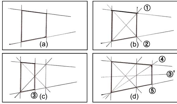
Figure 4: Depth measurement by the diagonal method: (a) initial perspective square, (b) sketching diagonals, (c) subdivision in half, (d) extension double.
