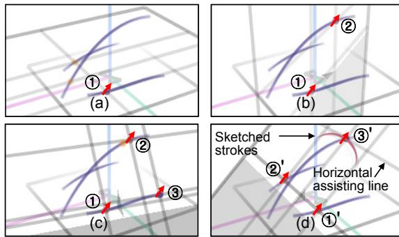
Figure 8: Tick-based sketch plane definition: (a) horizontal plane, (b) rotated vertical plane, (c) oblique plane, (d) sketching a continuous symmetric curve with a help of assisting lines.
