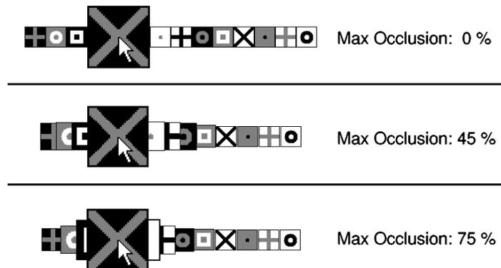
Fig. 10. In this design, limited overlap is allowed between adjacent buttons which alleviates the problems caused by sideways motion in Figure 9. The *Max Occlusion* factor controls the amount of overlap between neighboring buttons.
