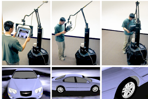
Figure 2: Navigating with the Boom Chameleon. When a user moves to the front of the space the front of the virtual car is viewable, moving to the side shows the corresponding side of the car, and moving closer to the center zooms to a close-up of the car.
