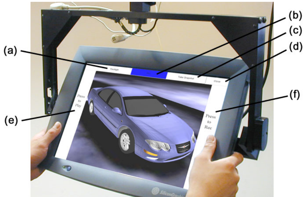
Figure 6: Annotation application hand grip and button layout. (a) Flashlight (b) Pen (c) Snapshot (d) Exit Application (e) Play (f) Record.
