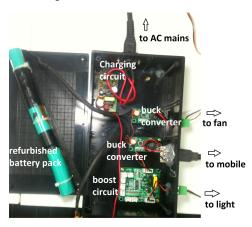
Figure 3: Component details of an *UrJar* prototype built using discarded laptop batteries.
