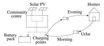
Figure 6: Illustration of system architecture
