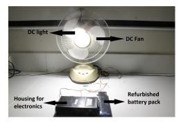
Figure 4: An UrJar prototype with DC appliances connected.
