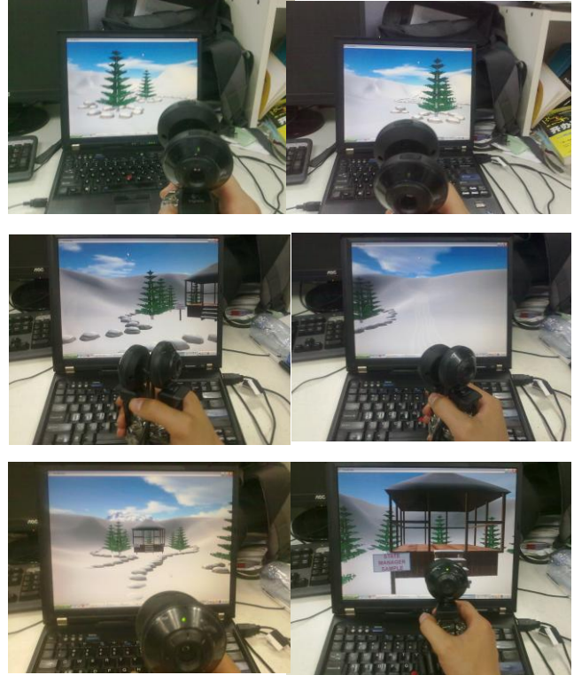
Figure 4. 3D navigation by using Back-to-Back. The first line shows: when user translates back-to-back to the left, the 3D scene also moves to the left. The second line shows that user rotates camera to the left. The third line shows when user pushes forward, the scene zooms in.
