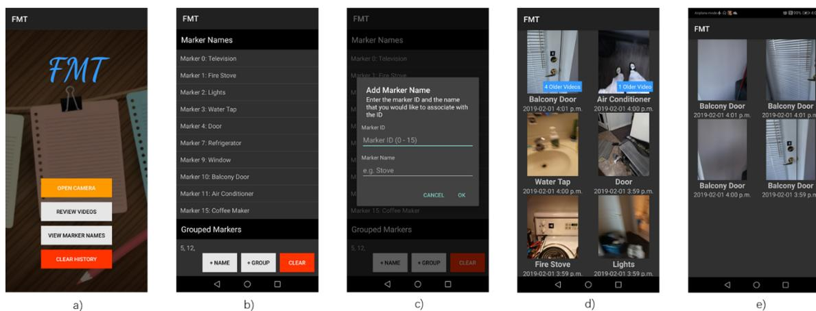
Fig. 3. The FMT application interfaces. (a) Home screen. (b) Interface to add, edit, or delete marker names and marker groups. (c) Pop-up dialogue to assign a name to a marker. (d) Interface to watch the recorded videos of tracked objects. (e) Older videos of the same objects.
