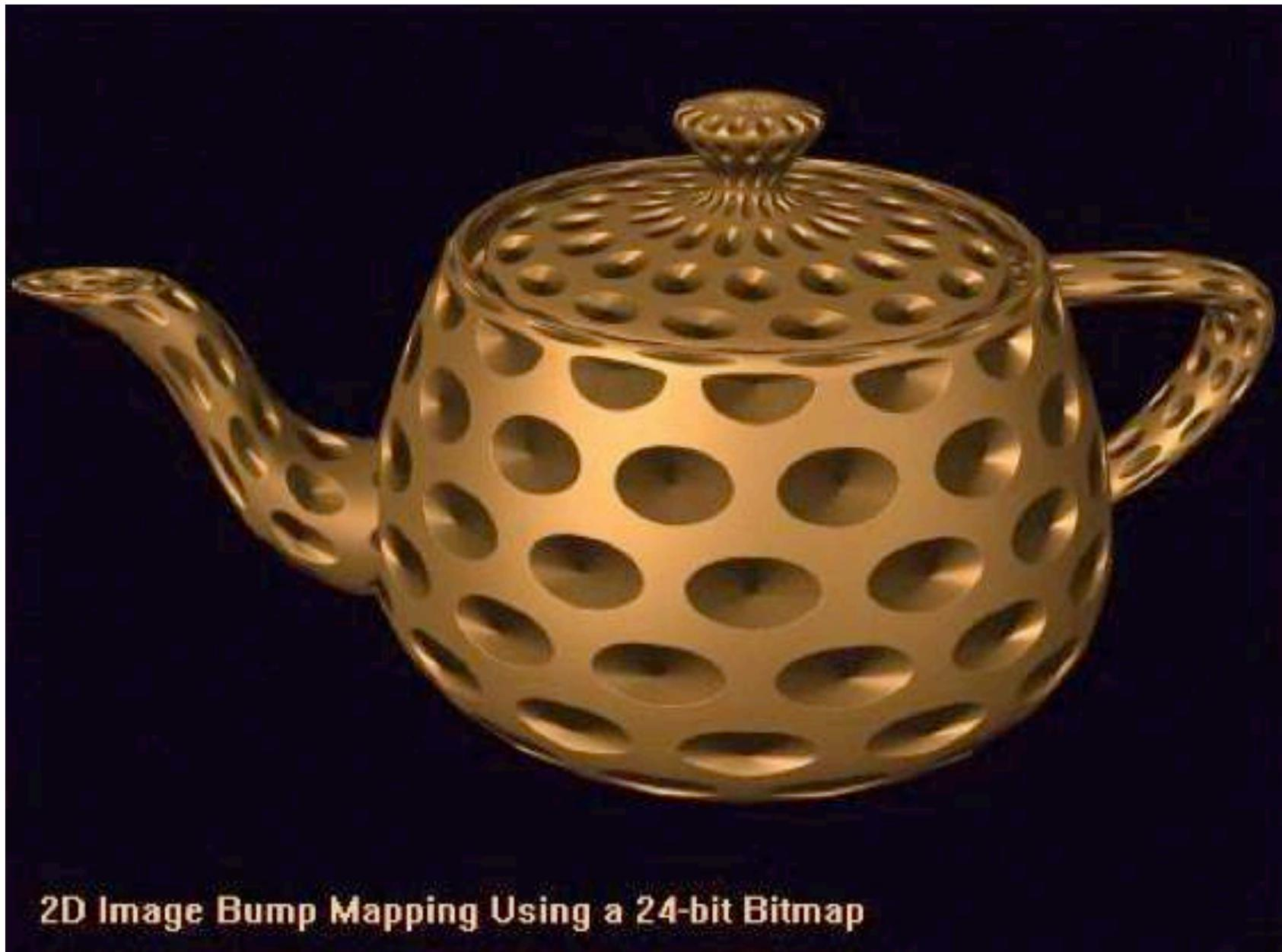
**2D Image Bump Mapping Using a 24-bit Bitmap**
