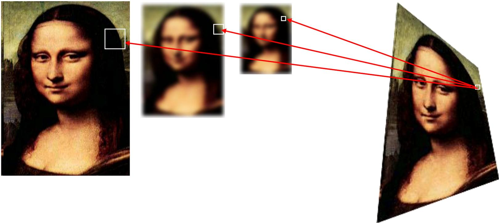
Given a polygon, use the texture image, where the projected polygon best matches the size of the polygon on screen.
