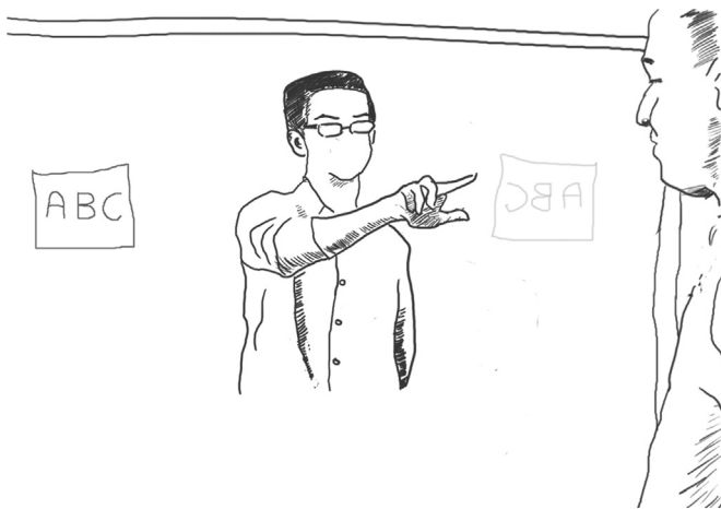
Fig. 9. The naïve two-projector solution, with unaligned graphics and bleed-through.
