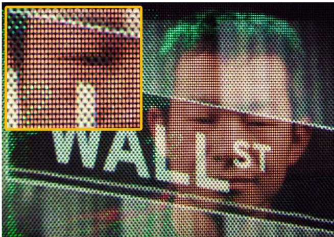
Fig. 12. The FACINGBOARD-2 open-weave projection screen.
