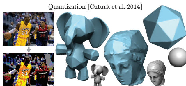
Fig. 15. Image quantization is applied to geometries and make surface patches facing toward pre-defined color palettes.
