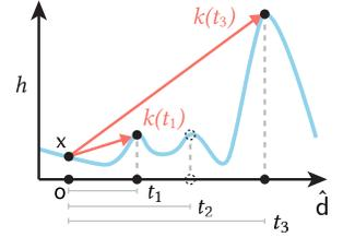
**Figure 6: We accelerate the computation by only searching for the discontinuities that have (primary) influence on the incoming radiance. For example, we ignore the peak at  $t_2$  because it is blocked by the peak at  $t_1$  and has no contribution to the incoming radiance.**
