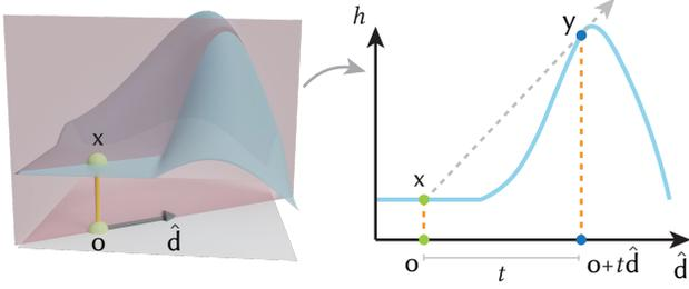
**Figure 4: Discontinuities in a heightfield are a subset of the peaks in a heightfield. We characterize a peak with respect to a point  $x$  with two conditions: (1) line  $x, y$  must be a tangent line at  $y$  and (2) the curvature of  $y$  along direction  $\hat{d}$  must be negative.**
