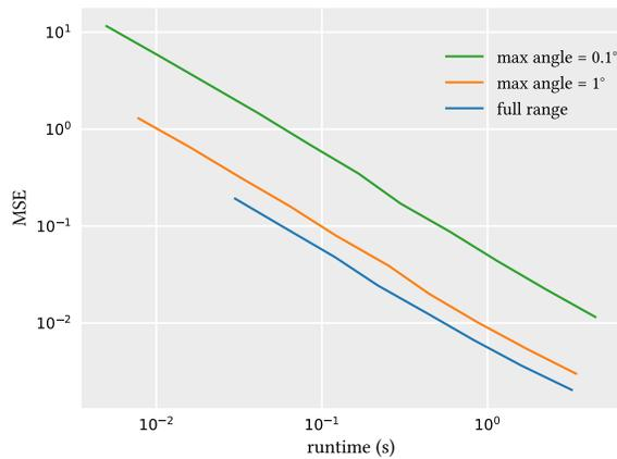
**Figure A4: We compare the variance vs time plot for different  $\theta$  search ranges. Full-range discontinuity searching (blue) provides the best numerical quality in gradient estimation at a cost of slowest per-sample performance. Reducing the search range (orange) can dramatically improve performance without introducing too much noise. Further reducing the search range can improve the performance even more at a cost of a much higher variance (green).**
