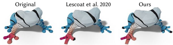
Fig. 15. By visualizing the biharmonic distance, we show that our approach can also postprocess the result from [Lescoat et al. 2020] (from 10,000 vertices to 800) and achieve better spectral preservation while still maintaining the same 1-ring sparsity pattern.
