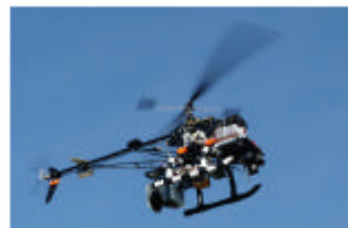
Figure 1: Instrumented helicopter platform. The system is based on the Bergen Industrial Twin, with a modified SICK LMS laser range finder, a Crossbow IMU, a Honeywell 3-D compass, a Garmin GPS, and a Nikon D100 digital camera. The system is equipped with onboard data collection and processing capabilities and a wireless digital link to the ground station.
