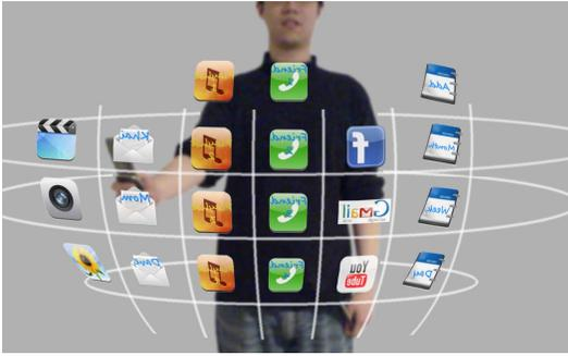
Figure 3: The layout of the Virtual Shelves used in the prototype evaluation.
