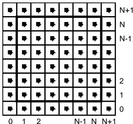
**Figure 2:** Computational grids considered in this paper. Both the density and the velocity are defined at the cell centers. The grid contains an extra layer of cells to account for the boundary conditions.
