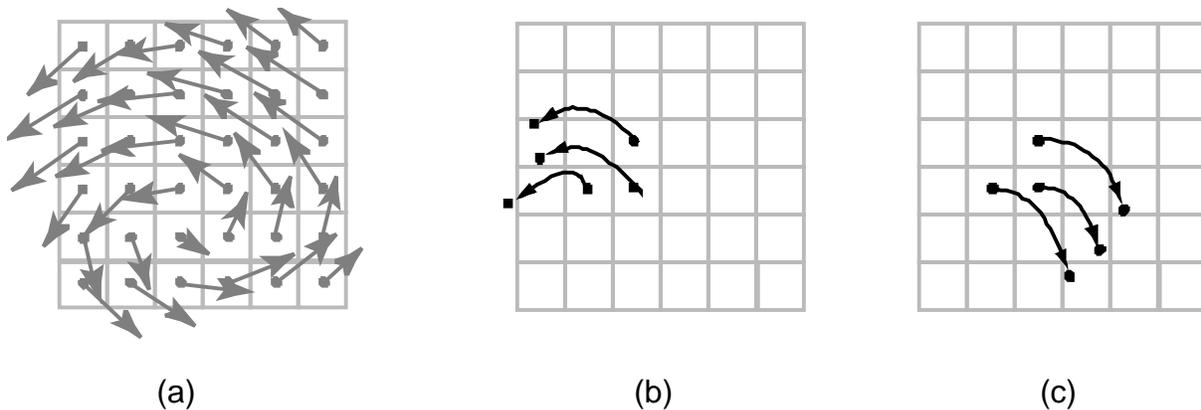
**Figure 6:** Basic idea behind the advection step. Instead of moving the cell centers forward in time (b) through the velocity field shown in (a), we look for the particles which end up exactly at the cell centers by tracing backwards in time from the cell centers (c).
