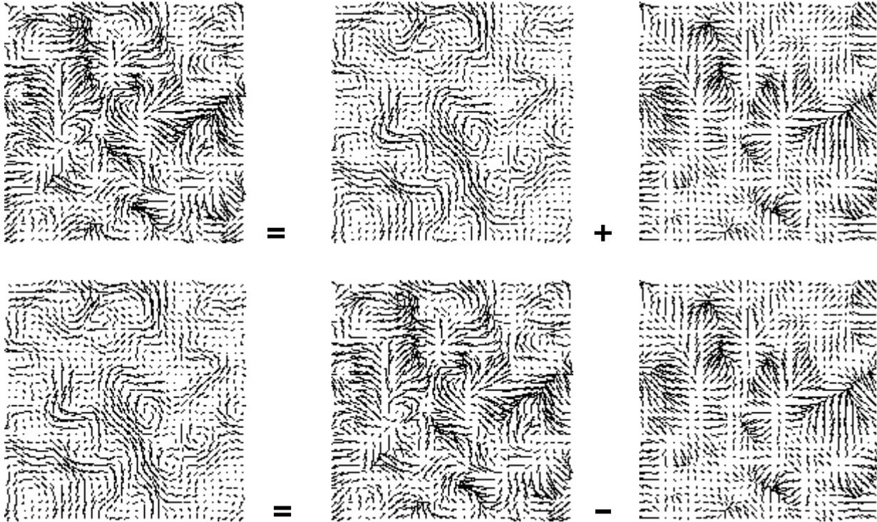
**Figure 7:** Every velocity field is the sum of an incompressible field and a gradient field (top). To obtain an incompressible field we simply subtract the gradient field from our current velocities (bottom).
