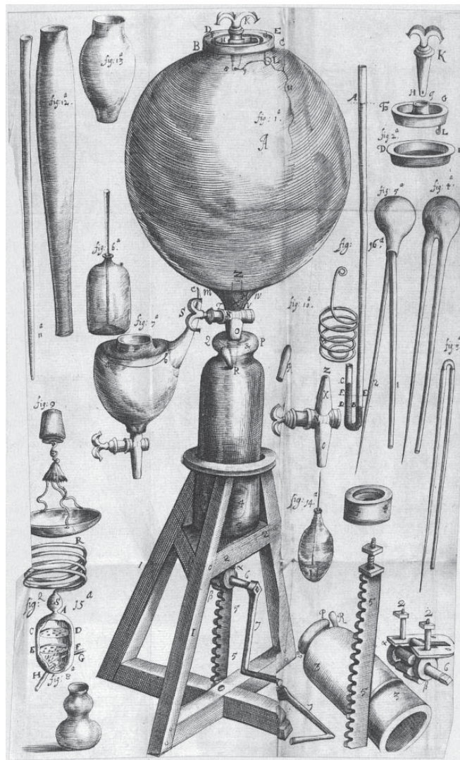
Boyle's air pump, which was constructed for his use by Robert Hooke in 1659, was a key piece of equipment in the experiments Boyle describes in his 1660 book New Experiments, Physico-Mechanical, Touching the Spring of the Air and its Effects . These experiments strikingly demonstrated the physical properties of air, showing that it had the capacity to exert pressure and to expand. This drawing of the pump was used to illustrate the book. From Boyle.
