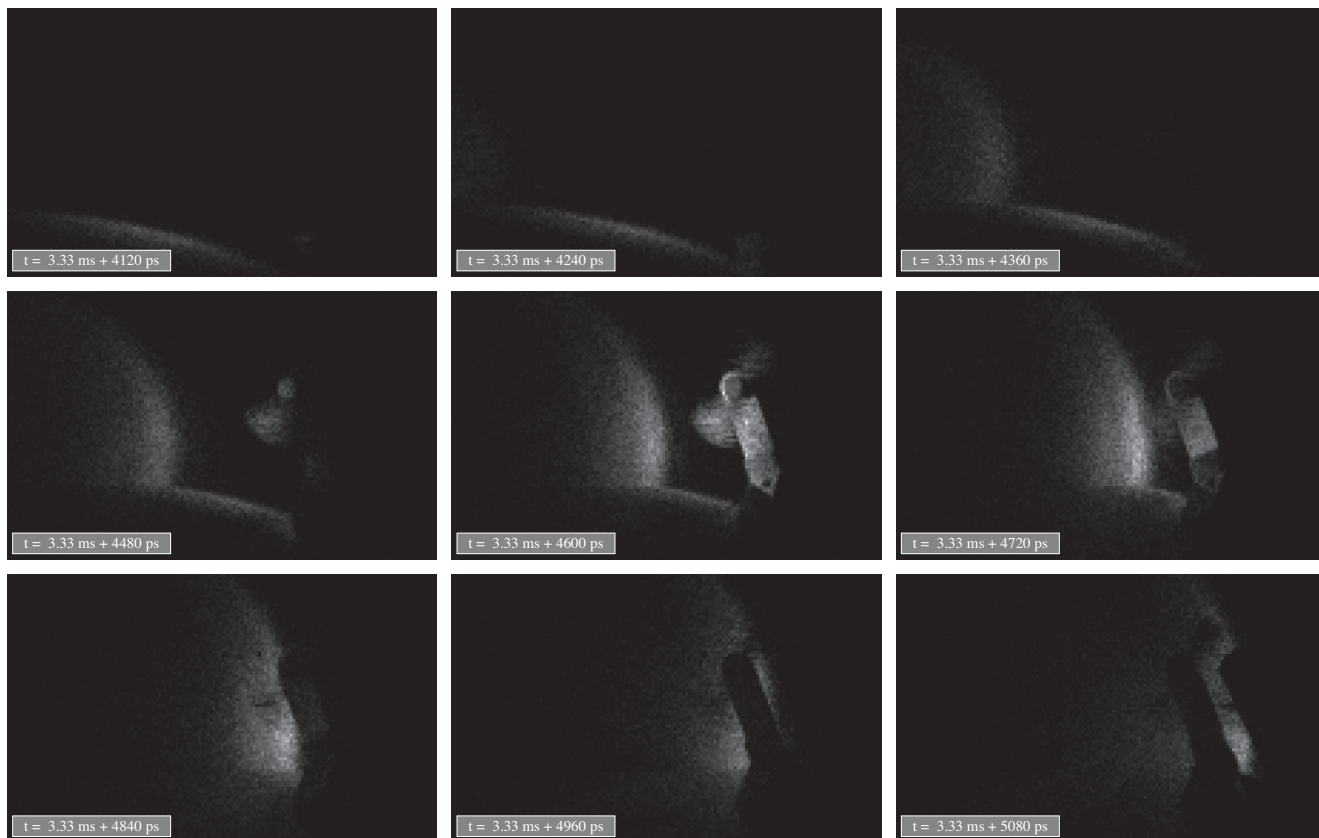
Figure 12: Images show a picosecond laser pulse propagating over two planes and a fan. Note how the fan blades appear as frozen. The effective frame rate is 250 Gfps.
