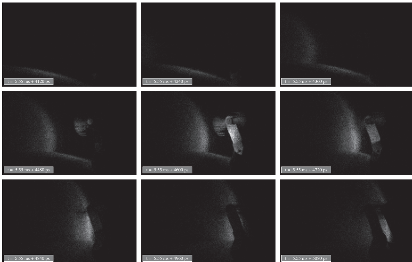
Figure 14: Images show a picosecond laser pulse propagating over two planes and a fan. The fan blades are at a different position demonstrating the unique capability of our approach to freeze time at all timescales .
