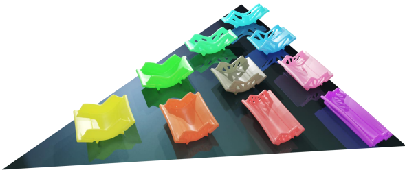
Fig. 2. Elastic eigenfunctions over Shape Space . With a single neural model, we can compute eigenfunctions for a bridge over the entire shape-space shown in Fig. 1.
