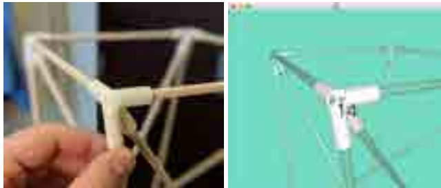
Figure 10: The joint geometries shown by RSAssembler match the 3D printed. Engraved joint IDs also facilitate orientation matching.
