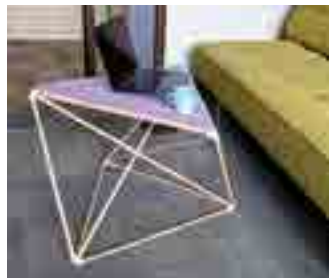
Figure 13: This tailored coffee table inherits the strength of hardwood dowels to supports not only itself, but also top panel and laptop (table in daily use for six months).
