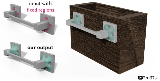
Fig. 27. Our variational formulation facilitates adding problem-specific constraints, such as constraining selected regions to stay put like these screw holes. See accompanying video for complete flow animation.
