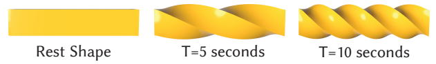
Fig. 10. This twisted beam example illustrates how our method handles large deformations in the presence of moving boundary conditions.
