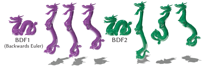
Fig. 11. Two dragons are simulated, one with an Implicit Euler time integrator (BDF1) and the other using BDF2. BDF2 produces a significantly less damped result.
