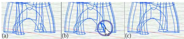
Figure 8: The existence of a global parametrization allows a user to quickly select an offending curve in a truss (a-b) and delete it to obtain the desired result (c).
