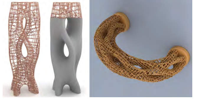
Figure 6: Our method works for arbitrary 3D shapes—independent of the homotopy class of the input mesh—as illustrated by these high genus examples. (Left) a genus-3 pillar is constructed by using our Michell Truss as the rebar skeleton before concrete is poured into the pillar shell. (Right) a high-genus input mesh is used to create a truss sculpture using metal bars. Input shapes created using Carlo Séquin’s Sculpture Generator ( https://people.eecs.berkeley.edu/~sequin/SCULPTS/scherk.html ).
