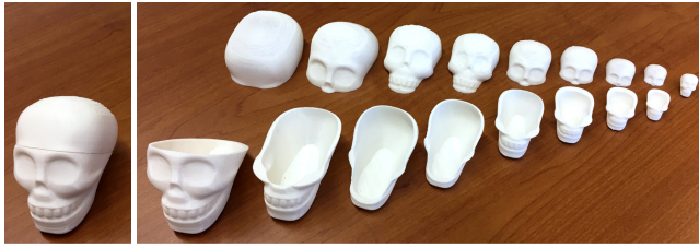
Figure 14: 3D printed Calaveras nest recursively. Each orientation and cut plane is determined automatically giving slight variations between layers. Our methods accommodate for printer tolerances, so nesting scale is determined at scale. Compared to the virtual result in Figure 5, an interesting polarity shift happens here: for smaller sizes, it is more efficient to nest upside down.
