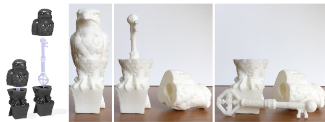
Figure 15: A “Glass Key” nests along an optimal removal direction within a “Maltese Falcon.”
