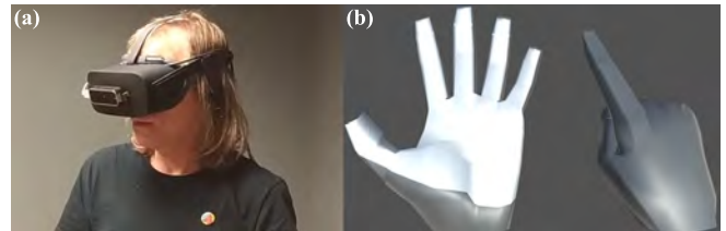
Figure 3. Experimental setup: Leap Motion mounted on an Oculus HMD (a), enabling participants to see their hands while gesturing (b).
