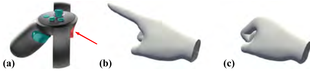
Figure 9. Touch-sensitive buttons and triggers on the Oculus Touch controller can be mapped to hand poses. For example, the absence of touch on the front trigger (a, red arrow) is interpreted as the index finger being extended (b), while its presence is interpreted as the finger being bent (c).
