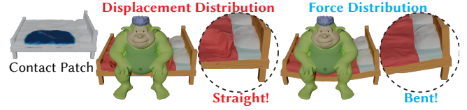
Fig. 8. A contact patch being used to specify a distribution on displacements results in an extremely localized deformation, deforming only the mattress as the ogre sits. Interpreting the contact patch instead as specifying a force distribution allows the resulting simulation to also capture global components of the deformation, such as the bending of the stiff frame Eq. (21). In this example, contact simulation is performed using a standard quadratic spring penalty with a single mode, and the ogre is approximated with a spherical collider.
