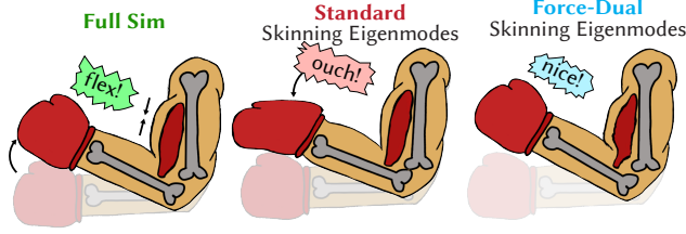
Fig. 11. We can generate subspaces well suited for heterogeneous material biomechanical muscle actuation. Standard skinning eigenmodes are not aware of the intended user interaction, and cannot accommodate the simulated flexing of the bicep without visual artifacts. Both simulations use four skinning eigenmodes.
