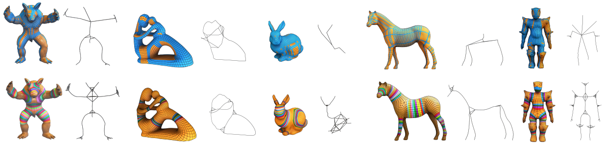
Fig. 6. Top row: in blue we see a single, particularly long face loop highlighted on meshes from Pietroni et al. Below: the FEQ face loops in regions covered by the blue face loop above are shown color coded.
