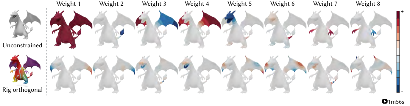
Fig. 6. We generate a linear blend skinning subspace for secondary motion parameterized by a set of skinning weights. Each weight i shown is independently normalized to lie between [-1, 1] \text{abs}(\mathbf{W}_i) and centered around 0. (Top) Weights generated by solving the unconstrained generalized eigenvalue problem on a weight-space elasticity Hessian. (Bottom) Secondary skinning weights that satisfy the weight-space complementarity constraint and are orthogonal to our rig space. These are naturally rig-aware, leading to higher frequency motion.
