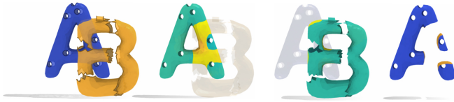
Fig. 12. Holey, non-manifold triangle meshes \mathcal{A} and \mathcal{B} each induce a generalized winding number function on the other’s faces, useful for boolean operations such as \mathcal{A} \setminus \mathcal{B} .
