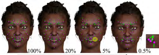
Fig. 10. UI layouts resulting from weighted random down-sampling of vertices. The UI layout created using 20% of the model vertices is qualitatively similar to the optimal layout (100%). Quality degrades with visual clutter at 5% and inter-element overlap at 0.5% down-sampling.
