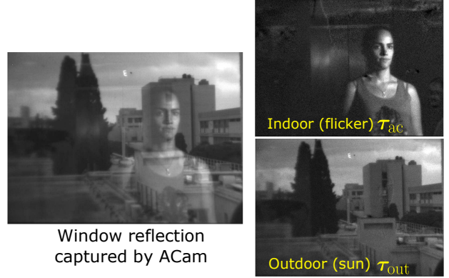
Figure 6. Temporal variations due to AC flicker are attributed to the indoor scene. ICA separates the indoor reflection from the transmitted scene. Both are recovered up to an unknown scale.
