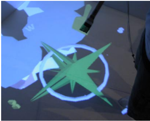
Figure 7 To rotate a painting, the user makes a circular gesture with the brush that activates this rotation widget.
