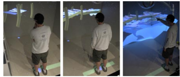
Figure 8 By moving around on a timeline widget placed on the floor of the Cave, an observer controls the state of the 3D painting currently displayed to see the artistic process that created the painting.
