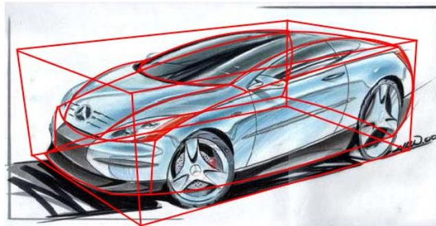
Figure 5. Simple 3D model creation for concept design
