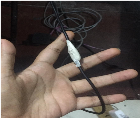
(a) Torn wire connected via soldering (covered with insulator) using academic knowledge (See 6.1.2)
