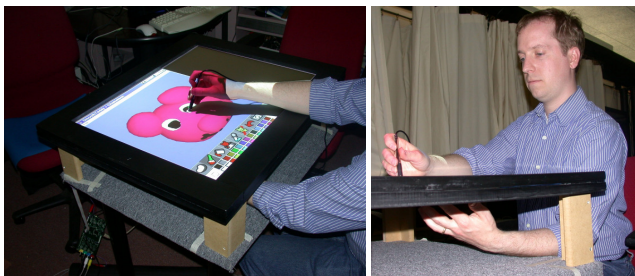
Figure 13. 3D object modeling and manipulation. Left: top-view of image being edited. Right: the user makes use of both hands simultaneously to draw and control orientation and position of the model.
