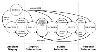
Figure 3. State diagram showing transition events between phases and states within phases.
