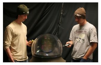
Figure 1. The prototype for our explorations allowed users to collaboratively interact with the volumetric display. Users' viewing positions and input devices were tracked in 3D.
