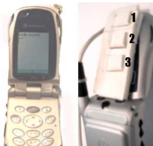
Figure 2. ChordTap prototype. The right image shows the chord keys mounted on the back of the phone.
