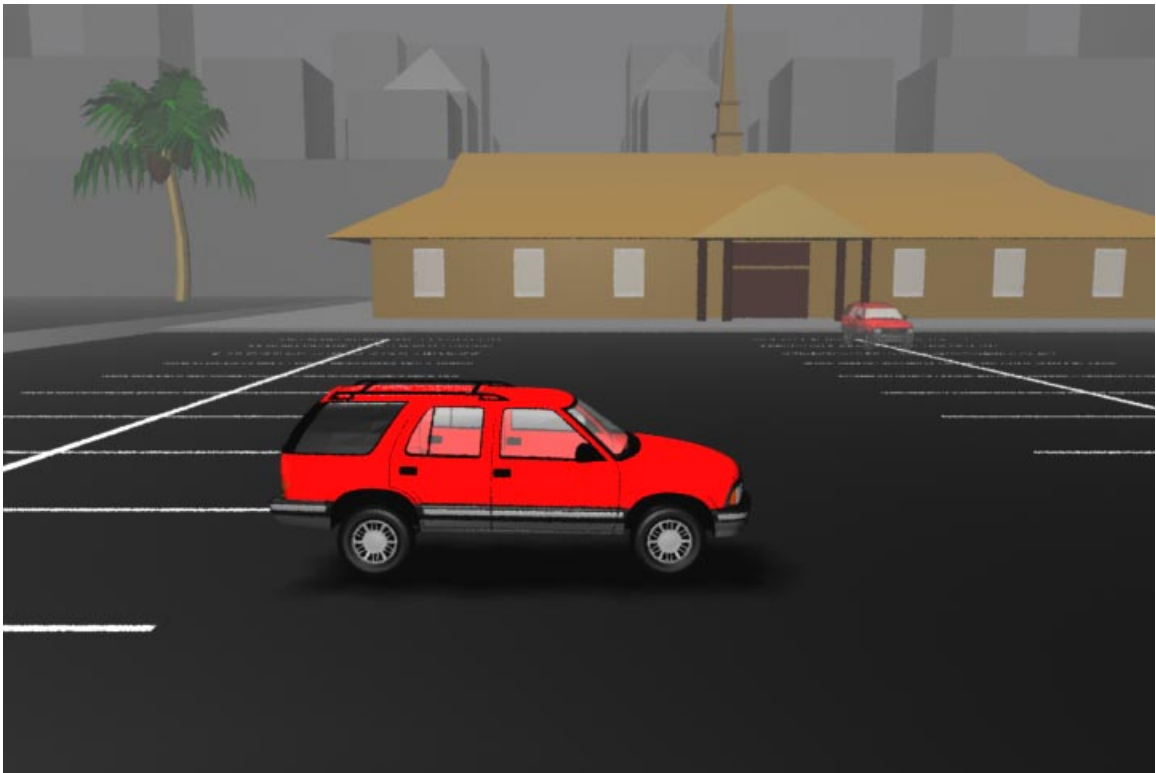
Figure E.2: The geometrical model of the truck. Underlying it is a physical model that consists of a rigid block that can slide on the plane z = 0 , and rotate around the z axis.
