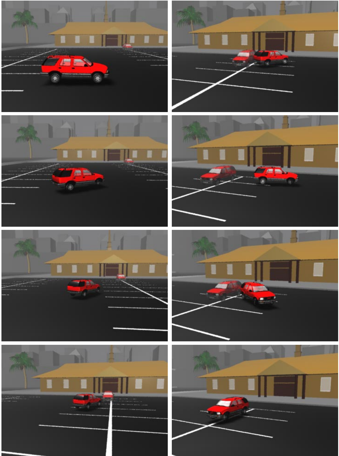
Figure 6.10: Frames from the animation showing the truck learning to park. The model far in the background indicates the desired position and orientation of the emulator at the end of the simulation.
