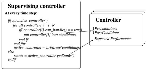
Figure 2: Controller selection and arbitration during simulation.
