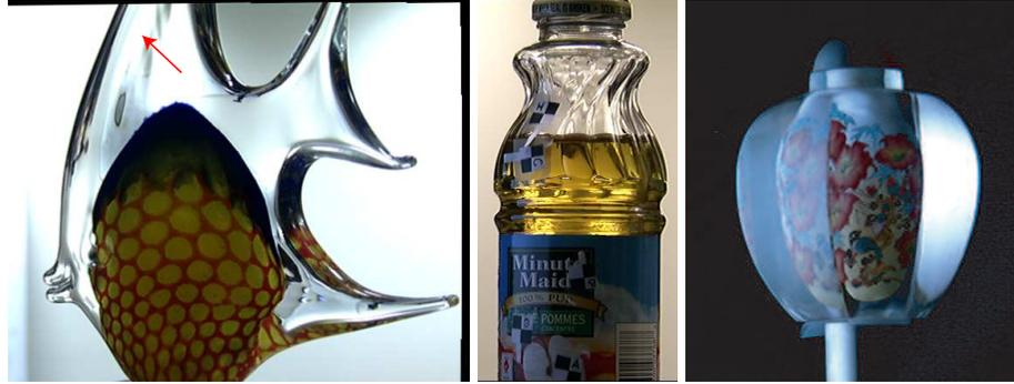
Figure 4.1: Three objects used in our experiments: A hand-made solid crystal sculpture with a painted interior (about 30cm tall), a partly-full juice bottle, and a decorative glass bottle with an opaque hand-painted interior. The red arrow highlights the pixel used in the example of Figure 4.16, bottom right.
