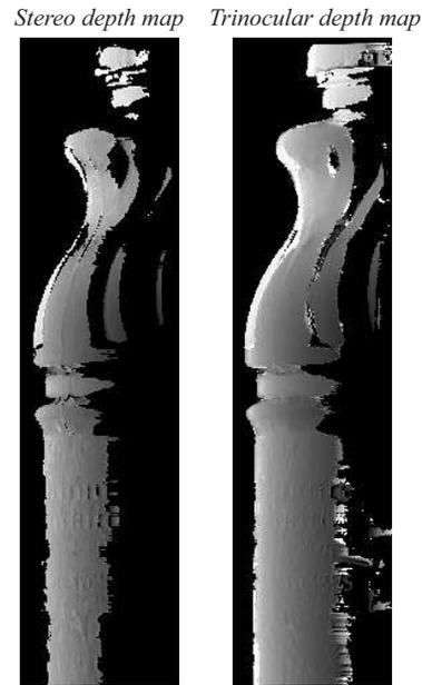
Figure 4.6: Juice reconstruction results. This figure also illustrates the improvement in reconstruction between two and three view reconstructions using the same reference view.
