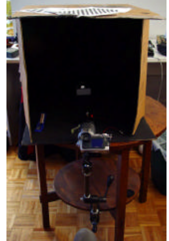
Figure 6: Apparatus used for bubble capture By conservation of energy the reflected light can be determined from the transmission fraction. This means the combined diffuse and specular reflective components must be (1-t) , so:
