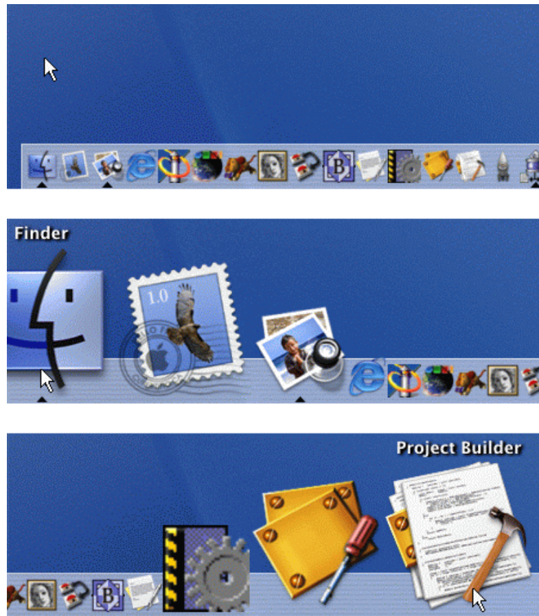
Figure 1.1: Screenshots of the “dock” in Mac OS X. ( Top ) When the mouse cursor is not over the dock, the icons are in an unmagnified, rest state. ( Middle and Bottom ) If the cursor passes over the dock, the nearest icons expand, and icons further away are pushed to the side.
