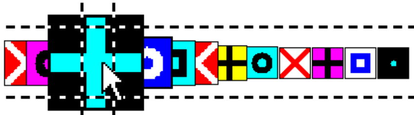
Figure 4.5: Dashed lines delimit a rectangle which the pointer must be within to acquire the button. Although the button looks larger than this rectangle, its full size is not available to the user: as soon as the pointer moves off the button’s centre, the button begins to contract.
