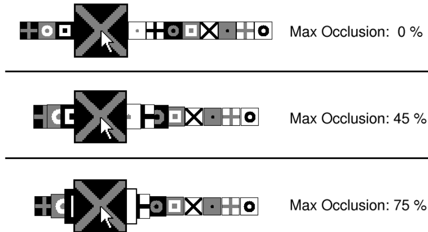
Figure 4.3: In this design, limited overlap is allowed between adjacent buttons, which alleviates the problems caused by sideways motion in Figure 4.2. The Max Occlusion factor controls the amount of overlap between neighbouring buttons.
