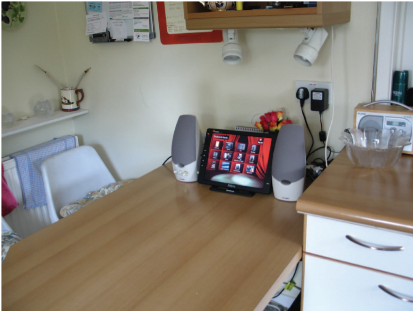
Figure 1. The Biography Theatre sits on Mr H's kitchen table and continually plays scenes from his past. The touch-screen interface allows users to select particular chapters, skip forwards and backwards through chapters, or pause the playback.
