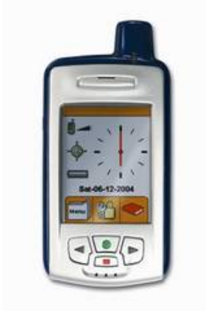
Figure 2.4: The Secufone offers GPS sensing in addition to telephony functions.
