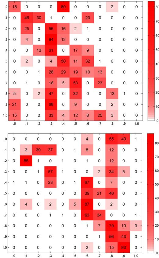
Figure 5. (Top) Confusion matrix of the classification results for the SVM model trained on data collected in standing upright orientation and tested on data collected in laid down orientation. (Bottom) Confusion matrix for the reverse case.
