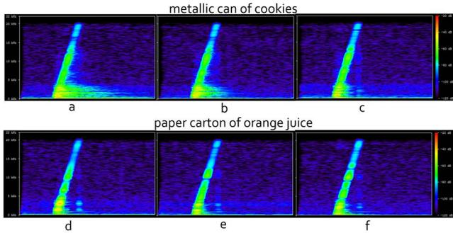
**Figure 1.** Spectrograms of impulse responses for 2 products (cookies, orange juice) in their original packaging when excited by a sine wave sweep at different content levels: empty (a, d), half (b, e), and full (c, f). The vertical axis is frequency and the horizontal axis is time. Color represents the intensity of sound.
