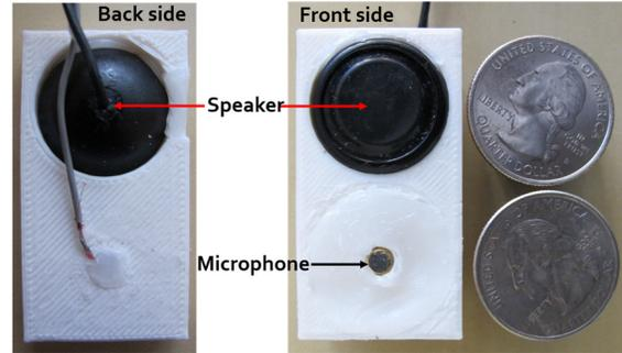
**Figure 2.** The SoQr sensor prototype which consists of a speaker and a microphone. When the sensor is installed on a container, the front side of the sensor (right) is placed to face and make contact with the container’s surface.
