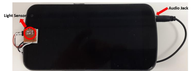
Fig. 3 To localize a phone, a light sensor is plugged into the audio jack of an android phone (Galaxy Nexus) for sampling the coded light in real time, which are then feed to a decoding algorithm.
