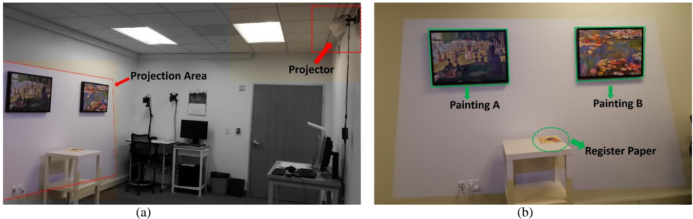
Fig. 7. Simulated mini Museum Environment Set-up in a room: (a) A projector is mounted on the top side of a wall and is projecting the coded light to the opposite side wall. (b) Two paintings are hang in the projection area and the museum registration paper is placed on a table.
